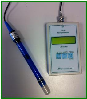
This digital pH-meter is robust and elegant of design and is accurate and simple in use. The temperature is automatic compensated (when temperature sensor is connected) and the instrument has an automatic calibration and data storage function which means that simplicity, and accuracy is guaranteed. The PH-95 is supplied in a handy carrying case with calibration liquids (pH-4, pH-7), user-manual and a storage liquid for the pH-electrode.
