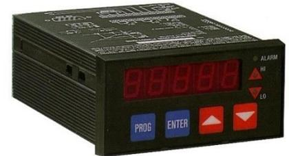
The HD9022 panel instrument is compact, versatile, precise and simple to program.
