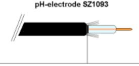
Take care, when stripping the cable, that the black carbon casing is stripped as far as possible. This otherwise can cause trouble during measements.
